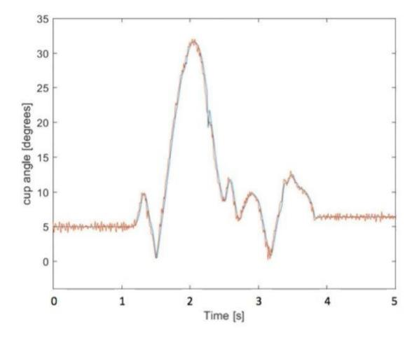
Figure 2: Example of cup angle series from inertial sensors (orange) and from an optoelectronic system (blue) during a sit to stand movement.
